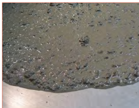
FIGURE 2: Concrete mix with 0.75 % sbwc of Exilva at initial spread
