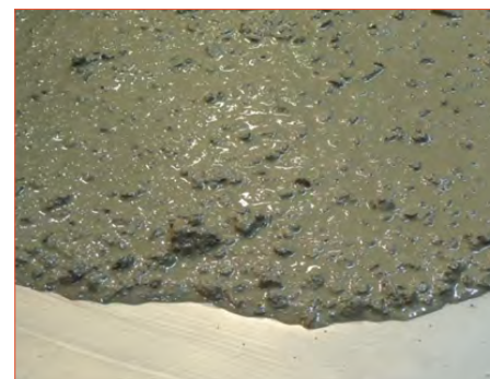
FIGURE 4: Concrete mix with 1.50 % sbwc of Exilva at initial spread
