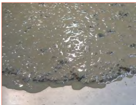
FIGURE 1: Reference concrete mix at initial spread
