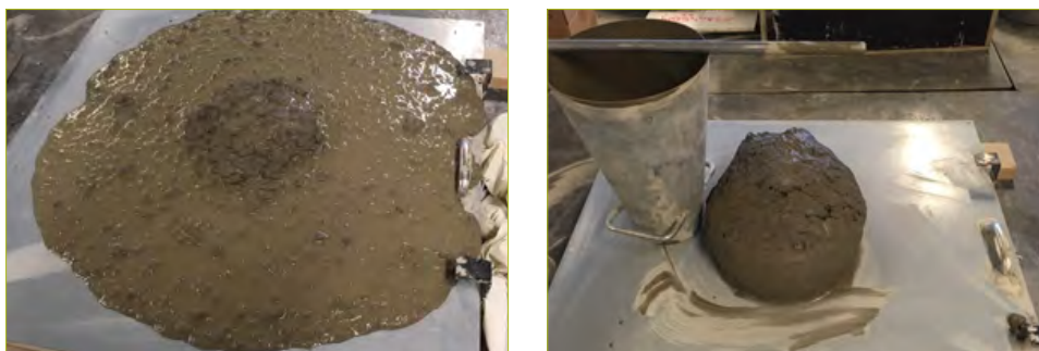
FIGURE 1: Visual Slump and Cone Results for the Reference (left) and Reference with Exilva P 01-L (right).
